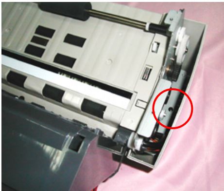
Remove one fixing screw on the right side
