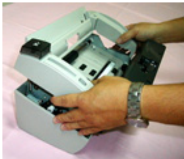
Remove the upper housing
