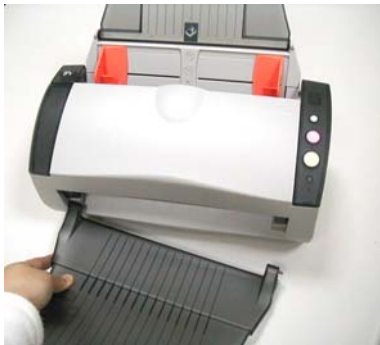
Press inwardly to remove the Output Paper Tray
