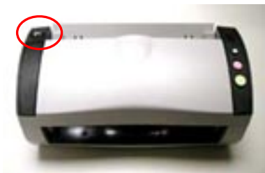
Press the ADF release button
