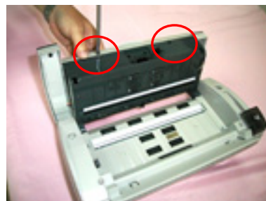
Remove 2 fixing screws
