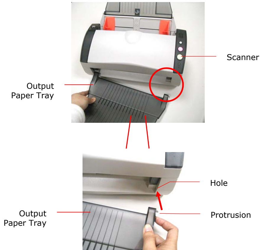
Figure 2.3 Installing the Output Paper Tray
