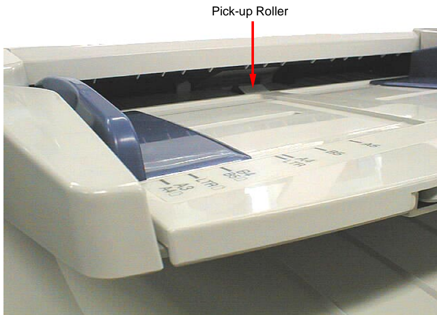
Figure 6-1. Pickup Roller Location
